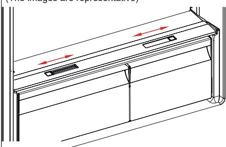
If the crisper is full, the fresh dial located in front of the crisper should be opened. This allows the air in the crisper and the humidity rate to be controlled, to increase the life of food within.
