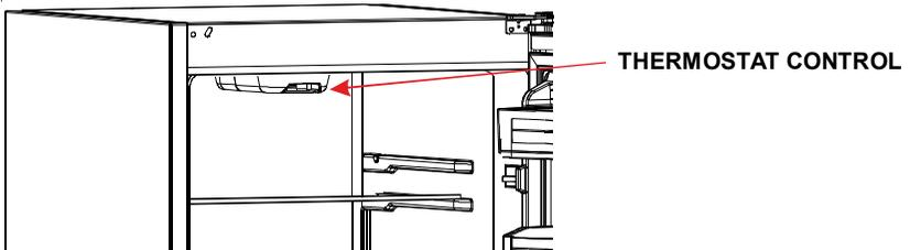
The fridge freezer thermostat automatically regulates the inside temperature of the compartments. By rotating the knob from position 1 to 5, colder temperatures can be obtained.
