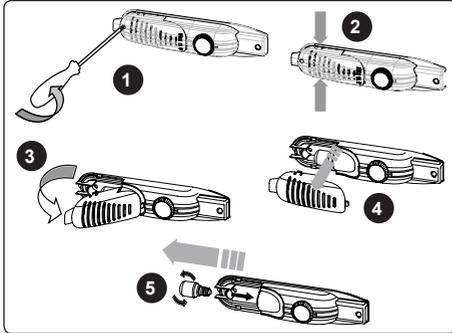
1. Remove the screw on the light cover by screw driver. (Fig.1)
