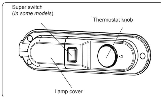
The fridge freezer thermostat automatically regulates the inside temperature of the compartments. By rotating the knob from position 1 to 5, colder temperatures can be obtained.
